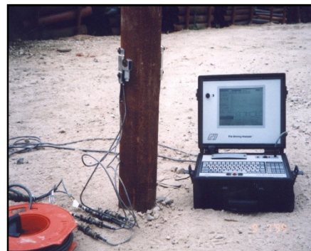
Dynamic load testing
