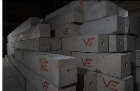
Cured beams numbered and stacked in the Van Elle factory waiting to be loaded onto a wagon in reverse order to be delivered to site.
