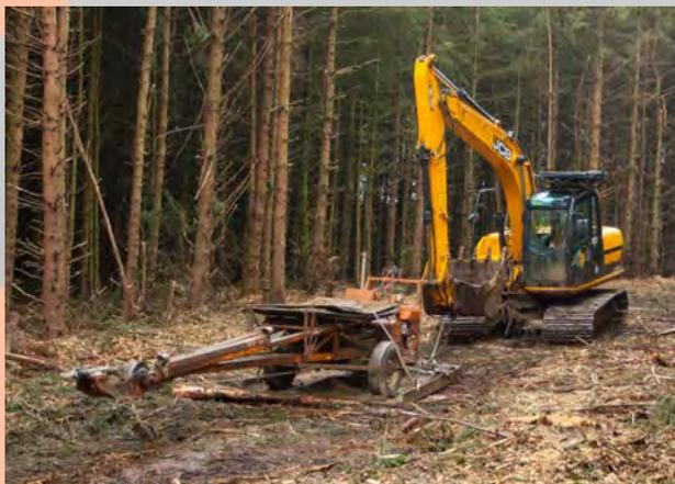
*Tripod rig towed safely on a metal skid*
