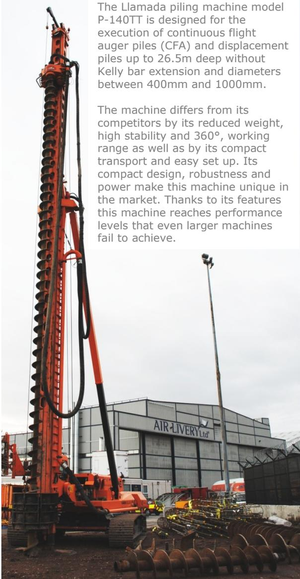
The Llamada piling machine model P-140TT is designed for the execution of continuous flight auger piles (CFA) and displacement piles up to 26.5m deep without Kelly bar extension and diameters between 400mm and 1000mm.
