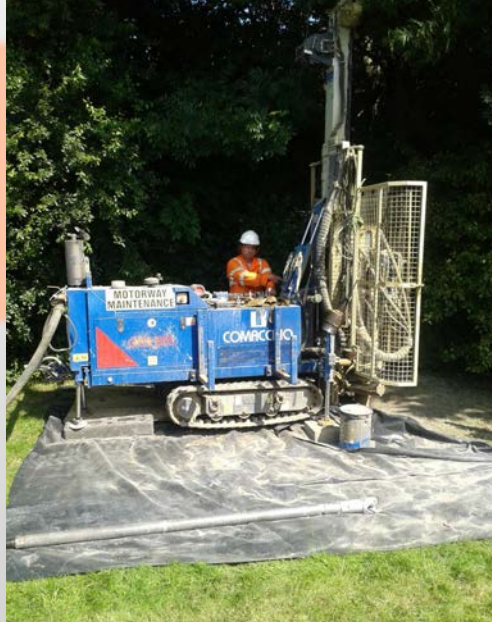
Comacchio MC205 being used for rotary drilling
