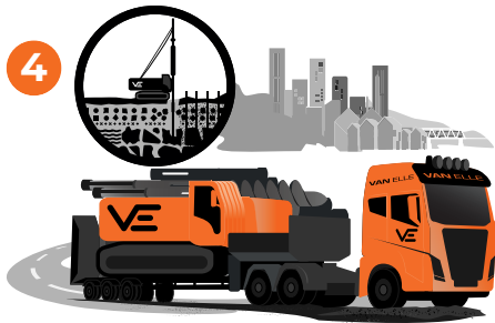
4 PILING as part of our package we can offer a range of piling techniques including continuous flight auger (CFA), pre-cast driven and tubular steel driven; constructing in-situ pile caps to bespoke designs
