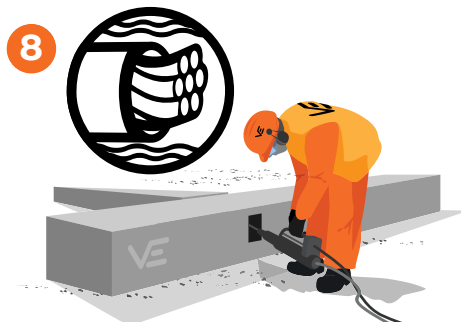
8 POST-TENSIONING we use a cable and hydraulics system with bitumen membranes to lock together the foundations creating an extremely sturdy single foundation unit
